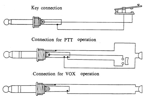
Ground lead for microphone should be wired separately and connected together to the ground lead of PTT switch at plug terminal.
